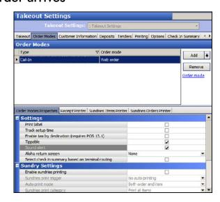
You can configure each ATO order type that is aligned with a POS order mode to play a sound when a new order arrives.
